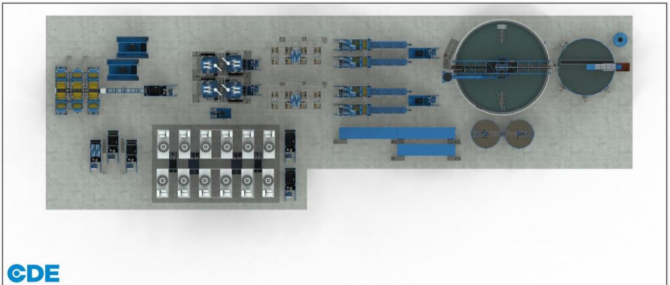
Figure 0-3 - Proposed NSP 5 Mtpa Processing Plant Layout
