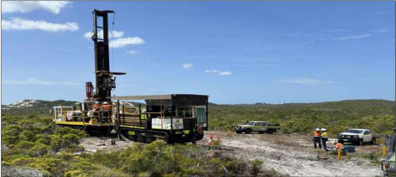
Figure 1: Sonic drilling rig completing groundwater bore drilling
