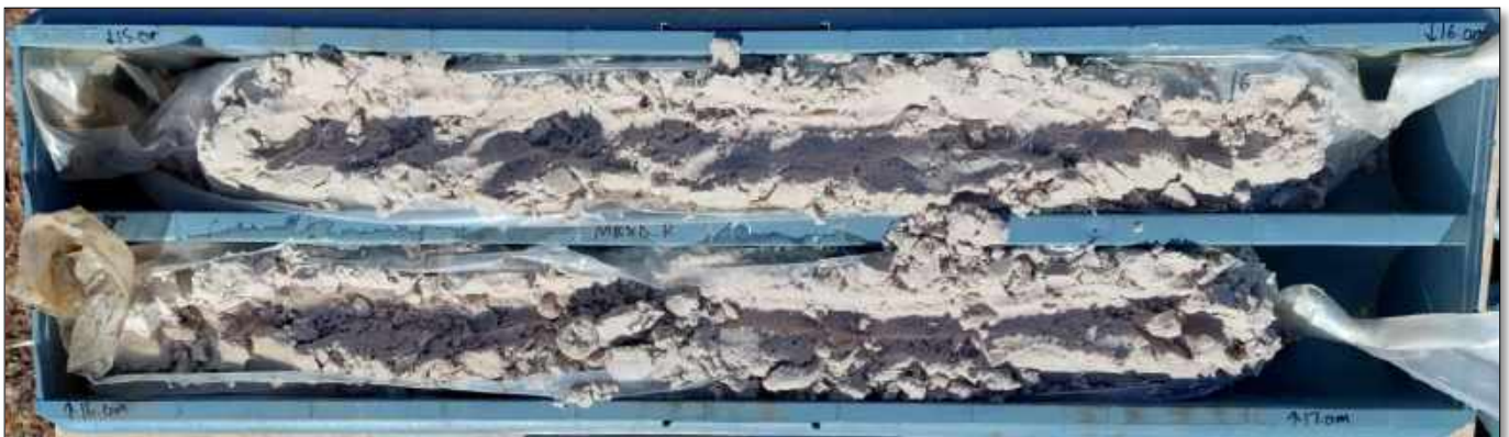
Figure 2: Silica sand core retrieved from sonic drilling
