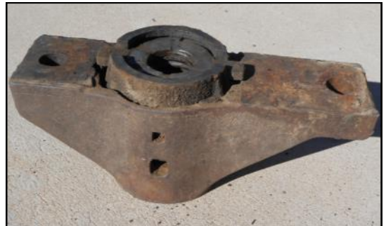
C. Removed compensator support, spring follower and springs still cemented together with historic dirt and grease.
