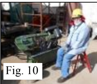
Fig. 10-11: George Trever is caught sitting down on the job, but he has a good reason. He is operating the metal saw to prepare staybolt sleeves. Though many of the staybolt components were purchased from suppliers in other parts of the country, there was much cutting, fitting and shaping work to be done on site. Fig. 12-13: In several instances, 2926 crew members had to come up with innovative solutions. In this case, flat copper washers were purchased and a tool was made to reshape them.
