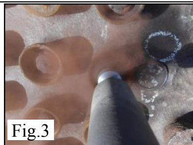
ALL staybolt assemblies must be cleaned, inspected and have a new copper sealing washer installed. Those components that are deteriorated beyond reuse must be replaced. Parts that are to be reused are cleaned and held for reassembly.
